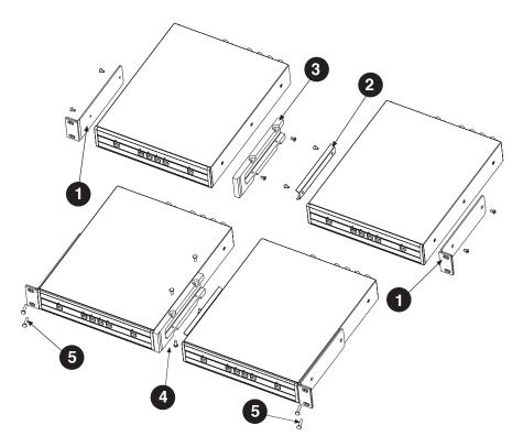
Figure 2. Double Mount (Quad Units Shown)
